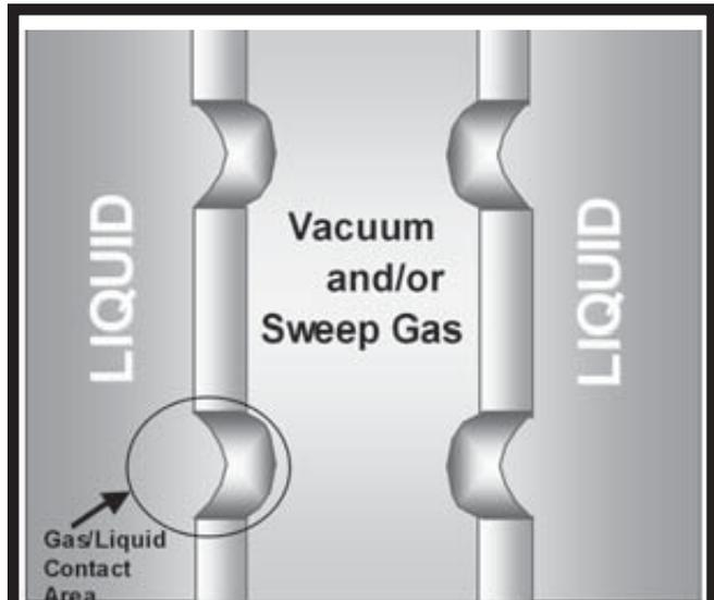
Figure 1. An illustration of pores in a contactor membrane.
