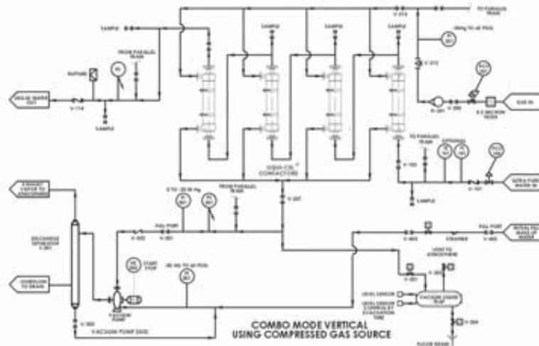
Figure 3. A typical piping schematic of a membrane system.
