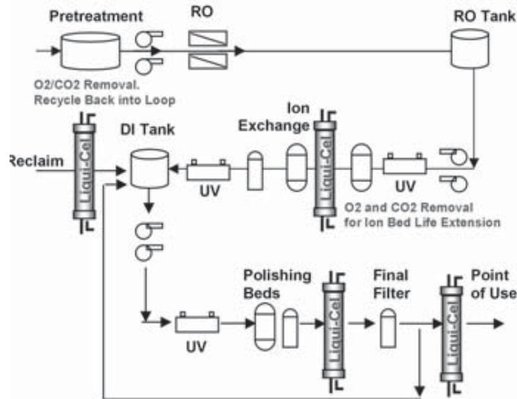
Figure 4. A basic layout for a typical high-purity water system.
